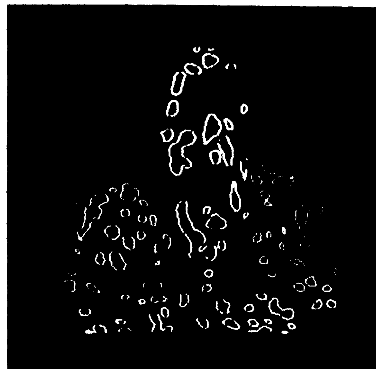
Fig. 9 The disparity map with disparity encoded as brightness
