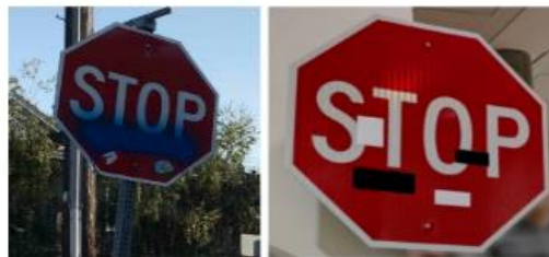
Fig. 2. Attacking stop signs with stickers[6]
