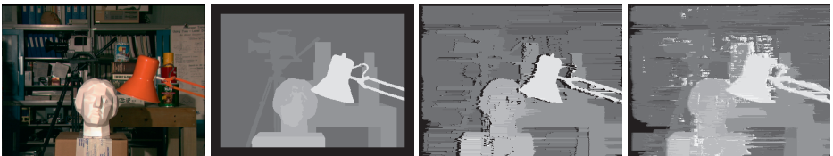
Figure 2: Three disparity maps for the Tsukuba image (Picture 1 from left). Picture 2 is the exact disparity map. Backtracking is used for Picture 3. The right disparity map (Picture 4) is calculated by finding the minimum element of each DP column.
