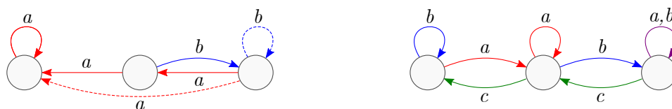
■ Figure 1 Two finite monotone co-Büchi automata recognising prefix-independent languages. For clarity, the co-Büchi transitions are not depicted but connect every pair of states; likewise, edges following from monotonicity (such as the dashed ones for example), are omitted. The automaton on the left recognises words with finitely many ab infixes. The automaton on the right recognises words with finitely many infixes in c(a^*cb^*)^+c .
