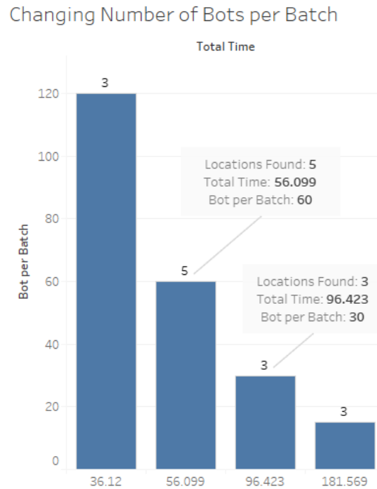
Figure 5.3: Results when running the test and altering the number of bots per batch.
