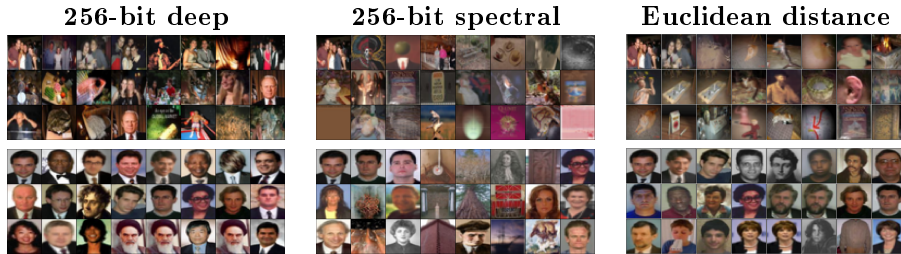
Figure 2: Retrieval results from the 1.6 million tiny images dataset using a full linear search with 256-bit deep codes, 256-bit spectral codes, and Euclidean distance. The top-left image in each block is the query image. The remaining images are the closest retrieved matches in scan-line order. The dataset contains some near-duplicate images.
