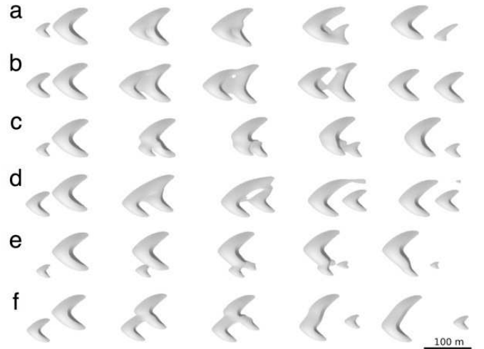
Figure 10: Snapshots of simulations of binary collisions for different values of \Delta and volume ratio r \propto (w/W)^3 . Calculations with r = 0.06 are shown for (a) \Delta = 0.2 , (c) \Delta = 0.6 and (e) \Delta = 0.9 ; calculations with r = 0.3 are shown for (b) \Delta = 0.2 , (d) \Delta = 0.6 and (f) \Delta = 0.9 .
