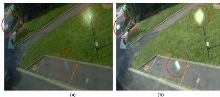
FIGURE 6. Nonsubsampled contourlet transform. (a) Using NSCT to directly fuse daytime background and nighttime frame. (b) Using NSCT to fuse daytime background and nighttime video frames from the result using improved framework for nighttime video enhancement, the algorithm can efficiently recover the unreasonable enhancement results due to imperfect moving objects extraction and to resolve some limitations of in [15].
