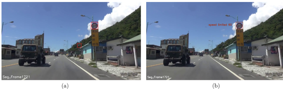
FIGURE 6. The incorrect road traffic sign image filtered result: (a) through road traffic sign detection, (b) after road traffic sign identification
