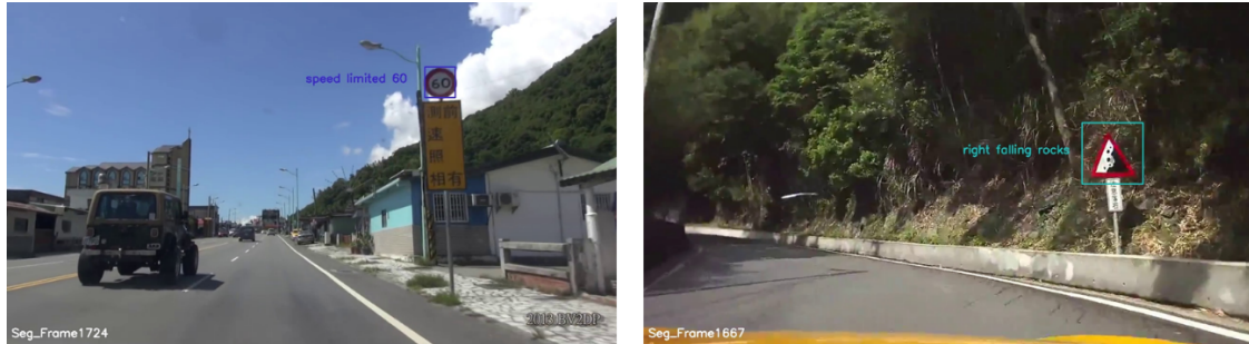
FIGURE 7. Recognition result: the left image shows the result of “speed limited 60” and the right image shows the result of “right falling rocks”
