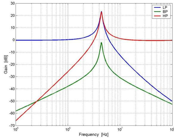
**Fig. 4. Magnitudes of current transfer functions,  $f_0 = 4.5$  MHz,  $Q = 20$**
