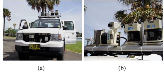
Fig. 1. a) The testbed vehicle and b) the sensors mounted on the roof.
