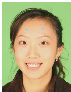
Figure 8.1: Two blue markers glued to the forehead are tracked and used as reference for the motion estimation.
