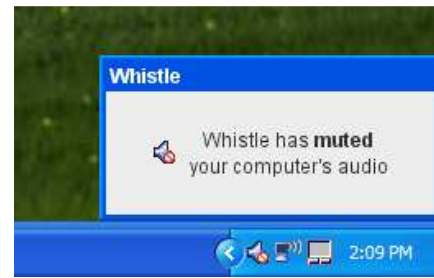
Figure 1. Whistle addresses the problem that people often forget to mute or unmute laptop computers. It collects a label each time a person manually toggles the mute flag, learning a relationship between context and a person's desired setting.
