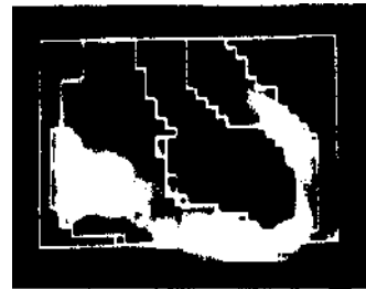
(F-2-3-4) Iterations of semantic region grower. The region grower used is grouping of all adjacent regions which are assigned the same meaning by the sequential assignment procedure, before the first assignment with low confidence level occurs. On each iteration the confidence threshold is lowered.
