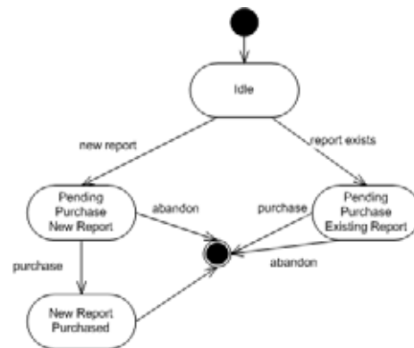
Figure 4. 'Billing' State Machine.
