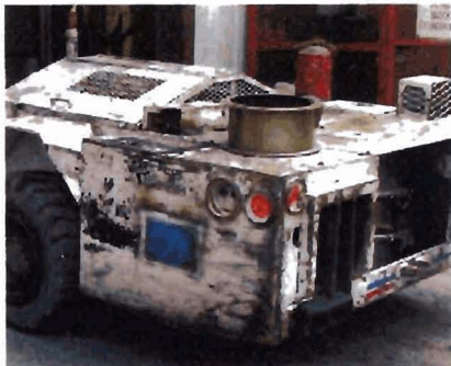
An extra ceramic filter will minimize downtime when dirty filters need to be regenerated.
