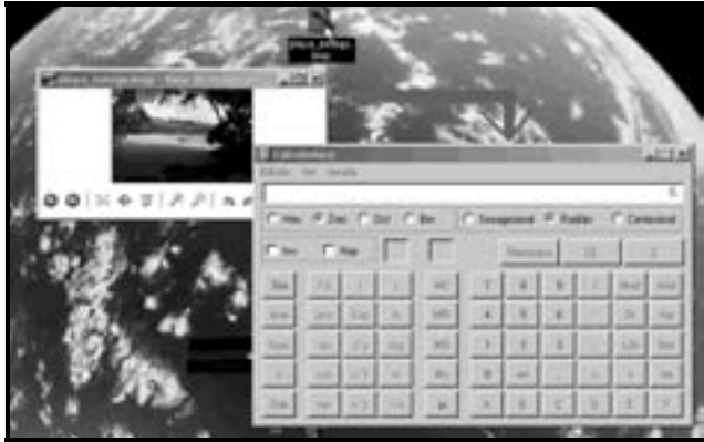
Fig. 7. Execution of calc.exe at the time visualizing 4 LSB steganographic image
