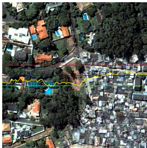
Figure 7. The adapted tile line (yellow) for the third example. Red and Green lines shows the buffer size (parameter t_2 ), and the Blue line shows the original tile line.
