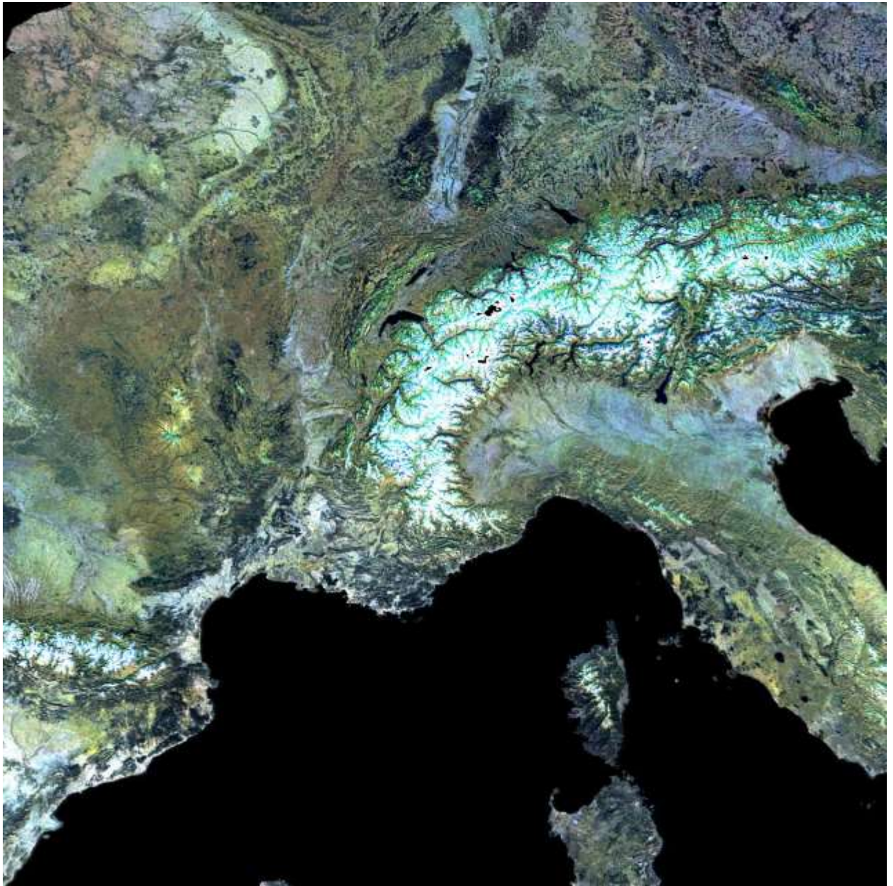
Figure 32-19. MODIS climatology VIS 'snow free' bihemispherical reflectance (white sky albedo) for (DOY 009, 041, 105 on RGB) scaled [0.016:0.128]
