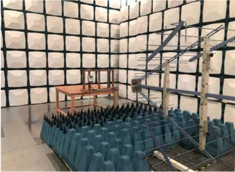
FIGURE 4.2 Experimental layout of electricity meter in 3m anechoic chamber
