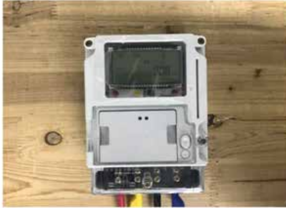
FIGURE 4.1 Prepaid single-phase electricity meter
