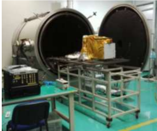
165 Fig.4. Thermal vacuum test of the EMI.
