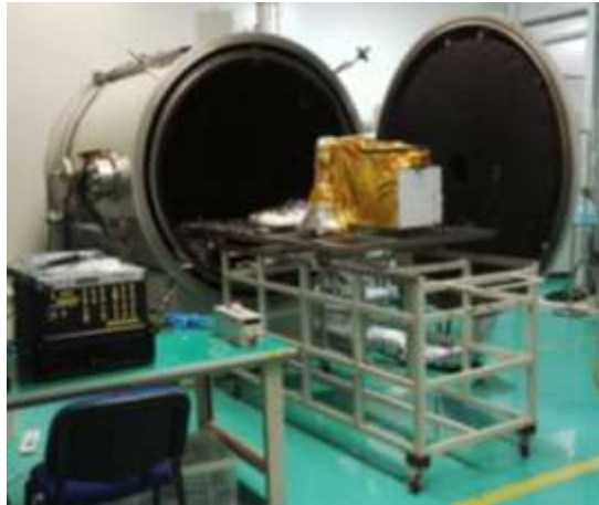
Fig.4. Thermal vacuum test of the EMI.
