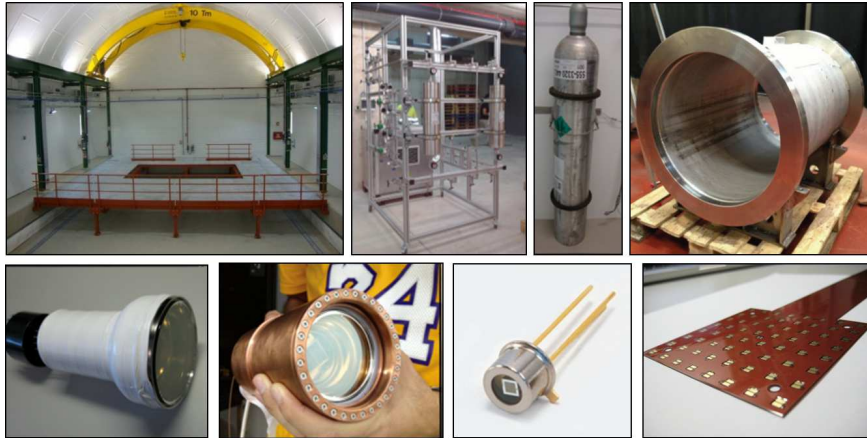
Fig. 4. Some relevant hardware components of NEW. From left-right, up-down: the platform supporting the experiment at Laboratorio Subterráneo de Canfranc (LSC), the gas system, 100 kg ^{136}\text{Xe} bottle, the vessel body, R11410-10 Hamamatsu PMT, PMT copper can, S10362-11-050P SiPM, piggy-tail SiPM board.
