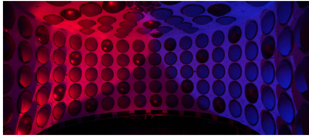
Figure 92. The interior of the CCM200 detector. Of the 200 PMTs, 80% are coated with wavelength shifter (TBP) to shift 128 nm scintillation light to the visible, leaving 20% uncoated (darker, more reflective PMTs in image), aiding discrimination of Cherenkov light. TPB foils cover the walls. The light-tight interior is surrounded by a veto region instrumented with PMTs. CCM is now running.
