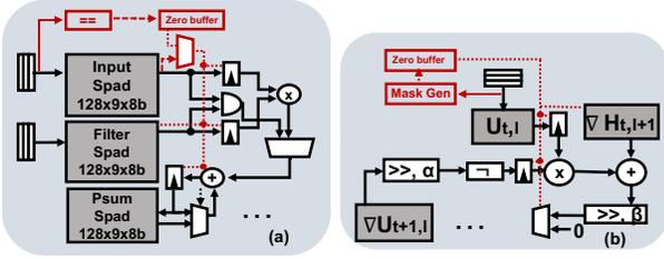
Fig. 6. Sparsity handling units inside PE and PGU. The red dash lines indicate the signal for sparsity handling units. We only show the units related to sparsity handling. (a) Leveraging input ( $S$  and  $\nabla U$ ) sparsity to save MAC and filter scratch pad reading. (b) Leveraging  $\nabla f$  sparsity to skip the related computations of  $\nabla S$ .
