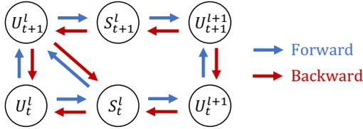
Fig. 3. Illustration of how BPTT works. During the forward propagation, the neuron of layer  $l$  at timestep  $t+1$  will retain the potential  $U_t^l$  and receive the spike  $S_t^l$  from the previous timestep, which is considered as the propagation in the temporal domain. In the spatial domain, the neuron at layer  $l+1$  receives the spike  $S^l$  from the previous layer. Forward paths are shown in blue arrows. For the backpropagation, the paths are reversed and shown in red arrows.
