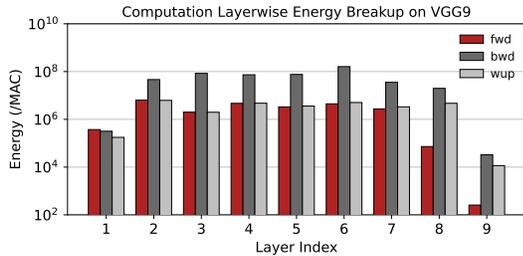
Fig. 15. Layerwise computation energy results on VGG9.
