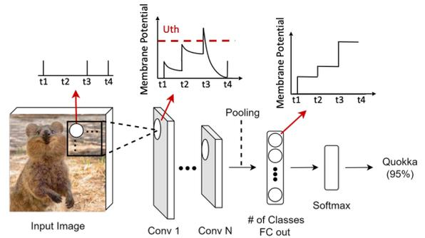
Fig. 1. An illustrative example of SNN. All intermediate neurons output rate-coded spikes and leak potential at each timestep  $t$ . Output neurons at the last fully connected layer will not generate spikes and only accumulate potential without leaking.
