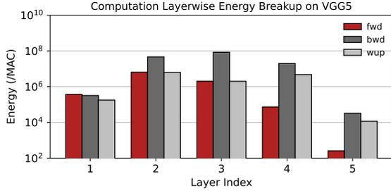
Fig. 9. Layerwise computation energy results on VGG5.
