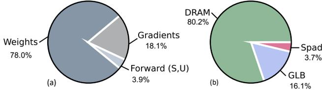
Fig. 10. Energy breakdown of the memory for VGG5 from the perspective of (a) algorithm memory components and (b) hardware memory components. In (a), the Gradients refer to the memory movement to calculate gradients ( $\nabla U$ ,  $\nabla H$ , and  $\nabla W$ ).
