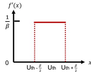
Fig. 2. Illustration of the curve to approximate the derivative of spike firing function. The derivative equals  $\frac{1}{\beta}$  when the membrane potential is inside the  $\beta$  range around the firing threshold  $U_{th}$  during the forward propagation and equals zero otherwise. We name  $\beta$  as the firing width.
