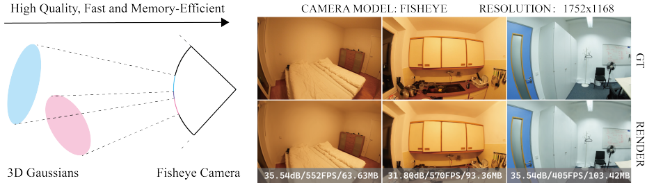
Fig. 1: Our Fisheye-GS. We have directly trained our 3DGS [13] model from images captured from fisheye cameras without undistortion to pinhole cameras. We then integrate our Fisheye-GS as a lightweight module within FlashGS [8], an efficient rendering technique for 3DGS, to evaluate its visual quality and performance.
