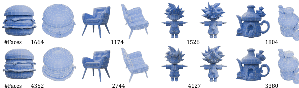
Figure 7: Coarse-grained face count control. Our model supports controlling the targeted number of face, which allows to generate meshes with different levels of detail.
