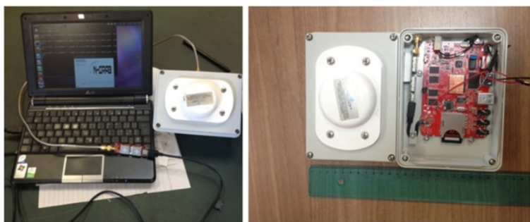
Figure 2 Prototypes of the GNSS-R receivers developed. PC-based solution (left panel). Hackberry board connected to the SiGe radio frequency front end (right panel).
