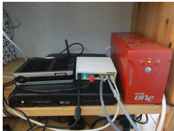
Fig. 3. Cloud resource at a community network node
