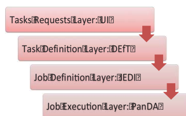
Fig. 6. Multi-layer architecture of the ATLAS production system for processing real and simulated data.
