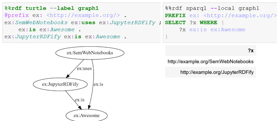
Fig. 2. Using Jupyter-RDFify: The left cell parses and visualizes an RDF graph given in Turtle format, the right cell queries the graph parsed from the left cell and outputs the variable bindings.
