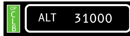
Figure 2: Representation of the OP CLB mode. When the aircraft has reached the altitude target, the OP CLB box disappears and the ALT mode is active, thus in green
