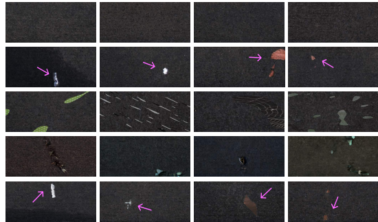
Figure 2: First row displays some negative samples from the KSDD2 dataset. The second row shows some images of positive samples from the same dataset. The third row shows the MemSeg-generated defect samples. The fourth row shows In&Out generated defect samples. Lastly, the final row showcases some images generated with DIAG. Notably, the defect images that DIAG generated are more realistic and in-distribution.
