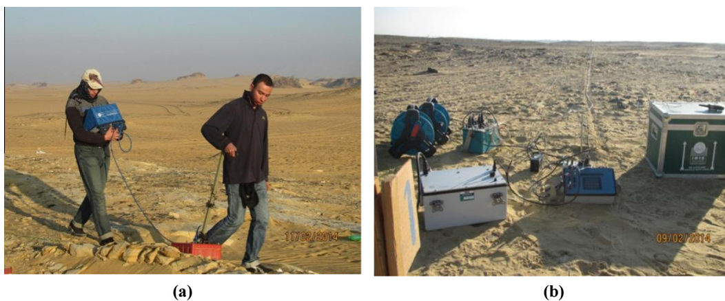
Figure 6 (a) Field photograph during the acquisition of GPR profiles, (b) Syscal R2 and multi-electrode system that used during the field survey.
