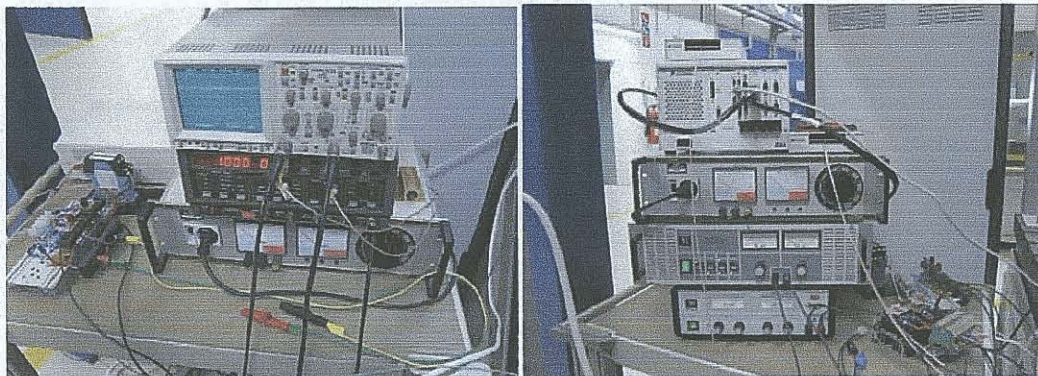
Fig. 113: Test rig equipment with function generator (left) and NI I/O card (right)
