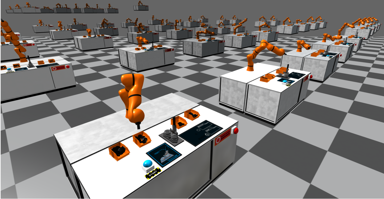
Figure 1-2.: The learning setup where the agents of 60 individual robots trained simultaneously the targeting of the respective components necessary for the collaboration procedure.
