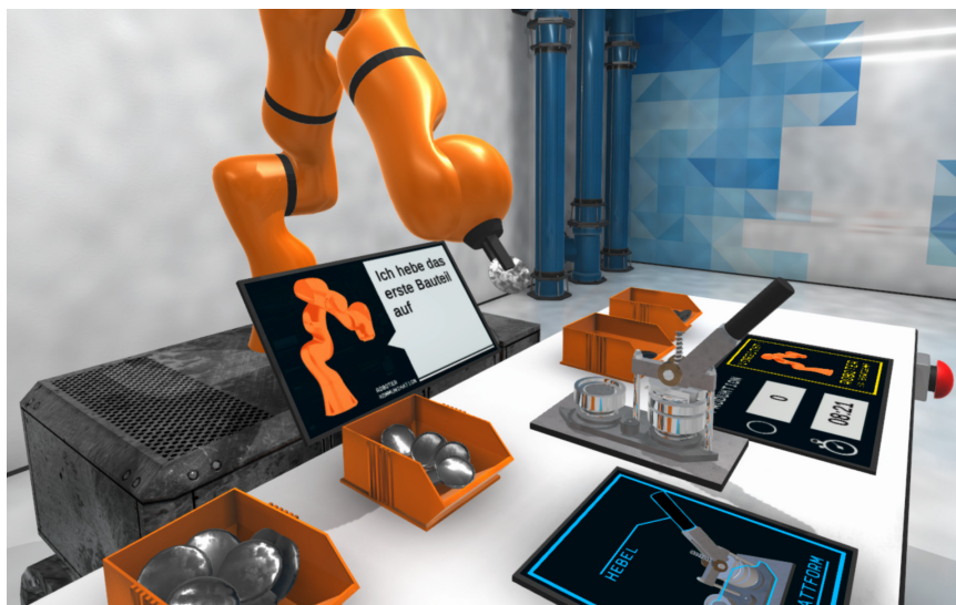
Fig. 2. The robot-arm extracts a component from one of the storage container while stating: “I pick up the first component”
