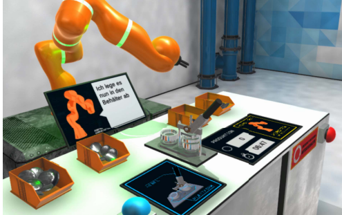
Fig. 1. The green light-signal emitted by the robot-arm indicating a correct operation. Below the text-panel where the robot-arm provides guidance and explanation to the participant.
