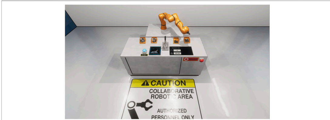
FIGURE 2 | The virtual workplace arrangement at which the participants conducted the shared task in collaboration with the robot arm. Apart from the pin-back button press and the container for the assembly components, the workplace contained a start and emergency shutdown button. Shown is the non-augmented condition where the three communication channels are absent. The virtual workspace where the shared task was executed by the participants in collaboration with the robot arm. The arrangement was designed Note that in the control condition the augmented communication channels are absent.
