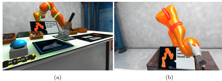
Fig. 5. The light-signal on the robot-arm: (a) green for operational, (b) red for collision or malfunction (Color figure online)
