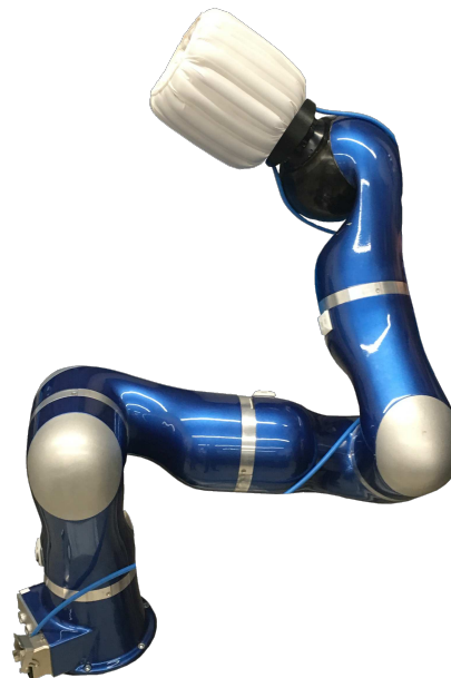
Fig. 1: The DLR Light-Weight-Robot - a sensitive torque controlled robot for safe human-robot collaboration equipped with a new module to ensure safety for all sort of tools.
