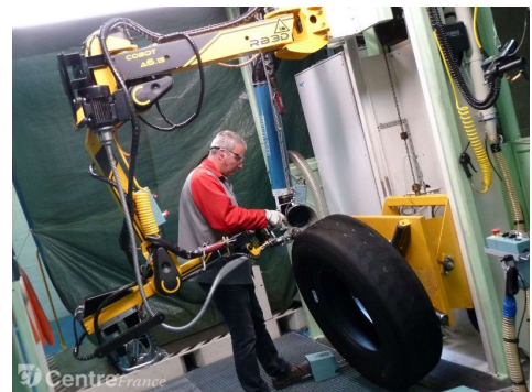
Figure 1: A collaborative robot providing strength amplification for tire retreading (developed by RB3D, CEA-LIST, CETIM).
