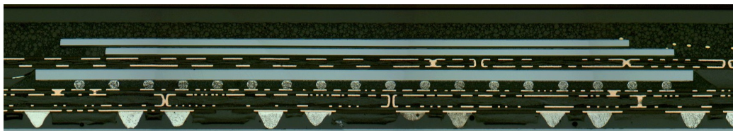
Figure 2: Cross-section of the A4 processor + RAM Package on Package (PoP) (taken from iFixit A4 teardown [ifi10])
