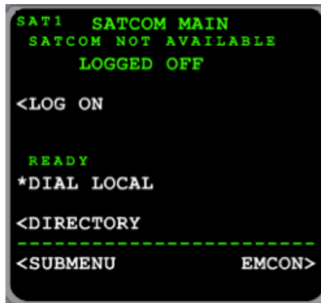
Figure 16: The SDU (Level D) Interacts with the MCDU ( Level A Component Present in the Cockpit)
