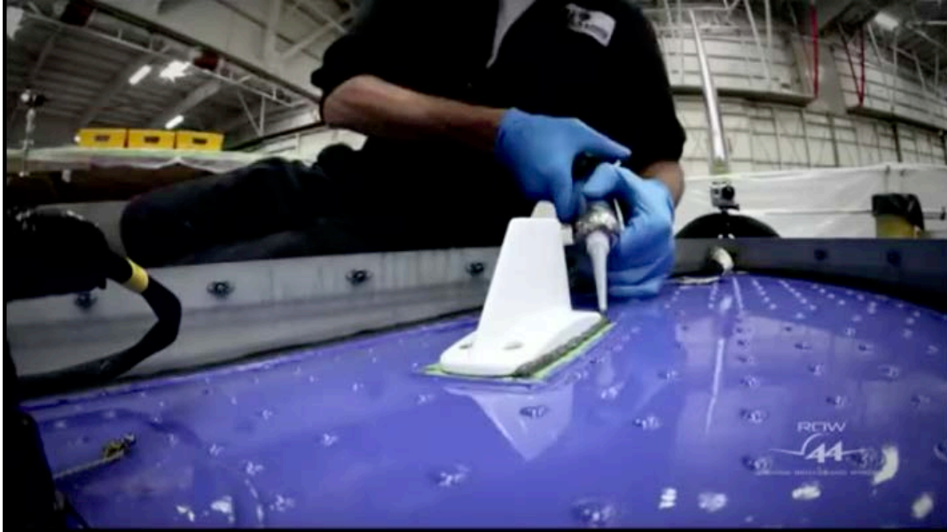
Figure 4. Cellular antenna in radome
