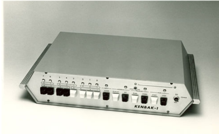
Figure 1.1: Kenbak-1, the world's first personal computer
