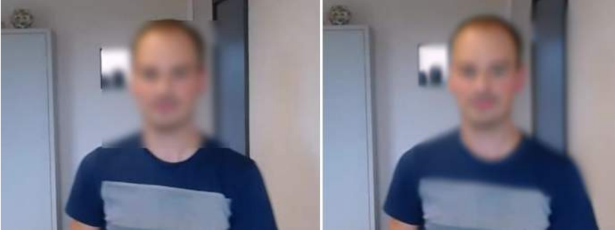
Figure 3.22: Blurring filters (left) standard Gaussian blur (right) smooth blurring filter.
