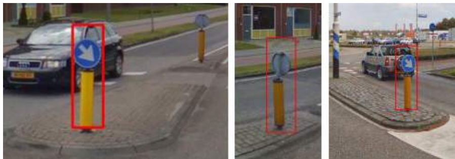
Figure 3.19: Example of the need for an extra filter for traffic signs still passing the post-processing steps.
