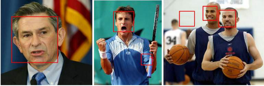
Figure 5.1: Example of CascadeClassifier.detectMultiScale() in OpenCV3.1 framework ( OpenCVBaseline model).
