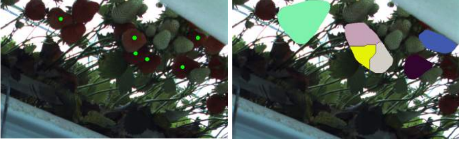
Figure 4.4: Watershed-based segmentation for separating object clusters.
