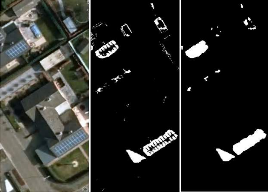
Figure 4.10: Example of pixel-based colour classification using shallow learning as the learning tool. (left) original image (middle) pixel classification result (right) cleaned up segmentation.
