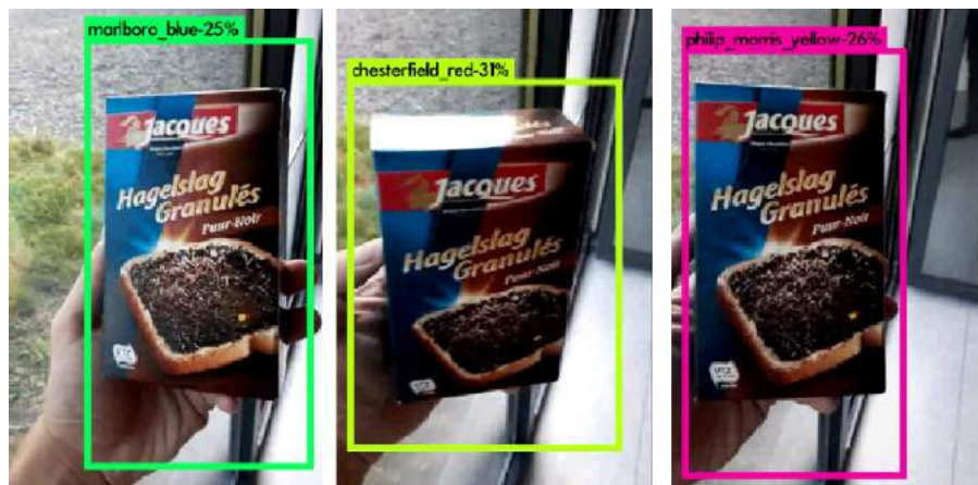
Figure 6.14: Detection triggered by our multi-class cigbox model on general rectangular boxes, like a box of chocolate chips.
