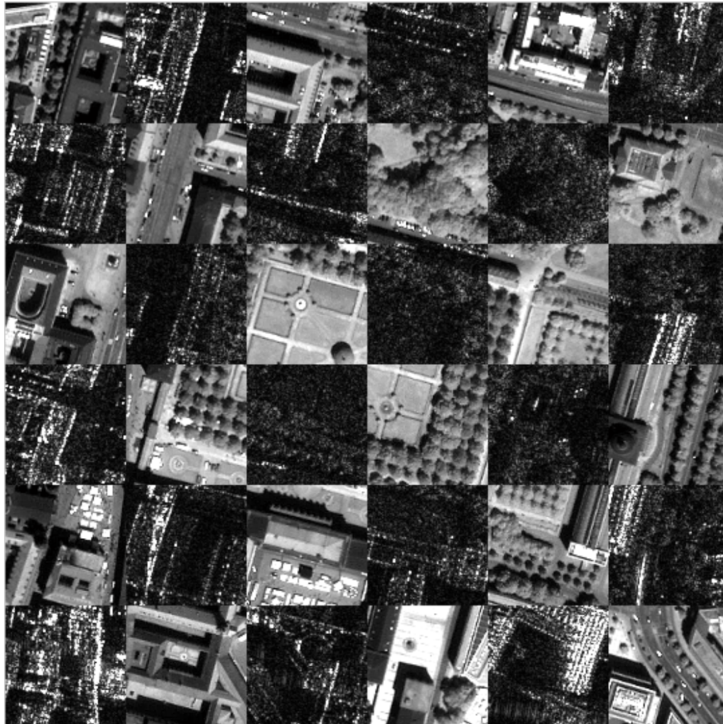
Figure 5.30: TerraSAR-X and orthorectified IKONOS through improved sensor orientation check squared to highlight good registration of “on ground” features like the park at the centre and the adjacent roads. Image area is of size 540×540 pixels and is displayed without any zoom.
