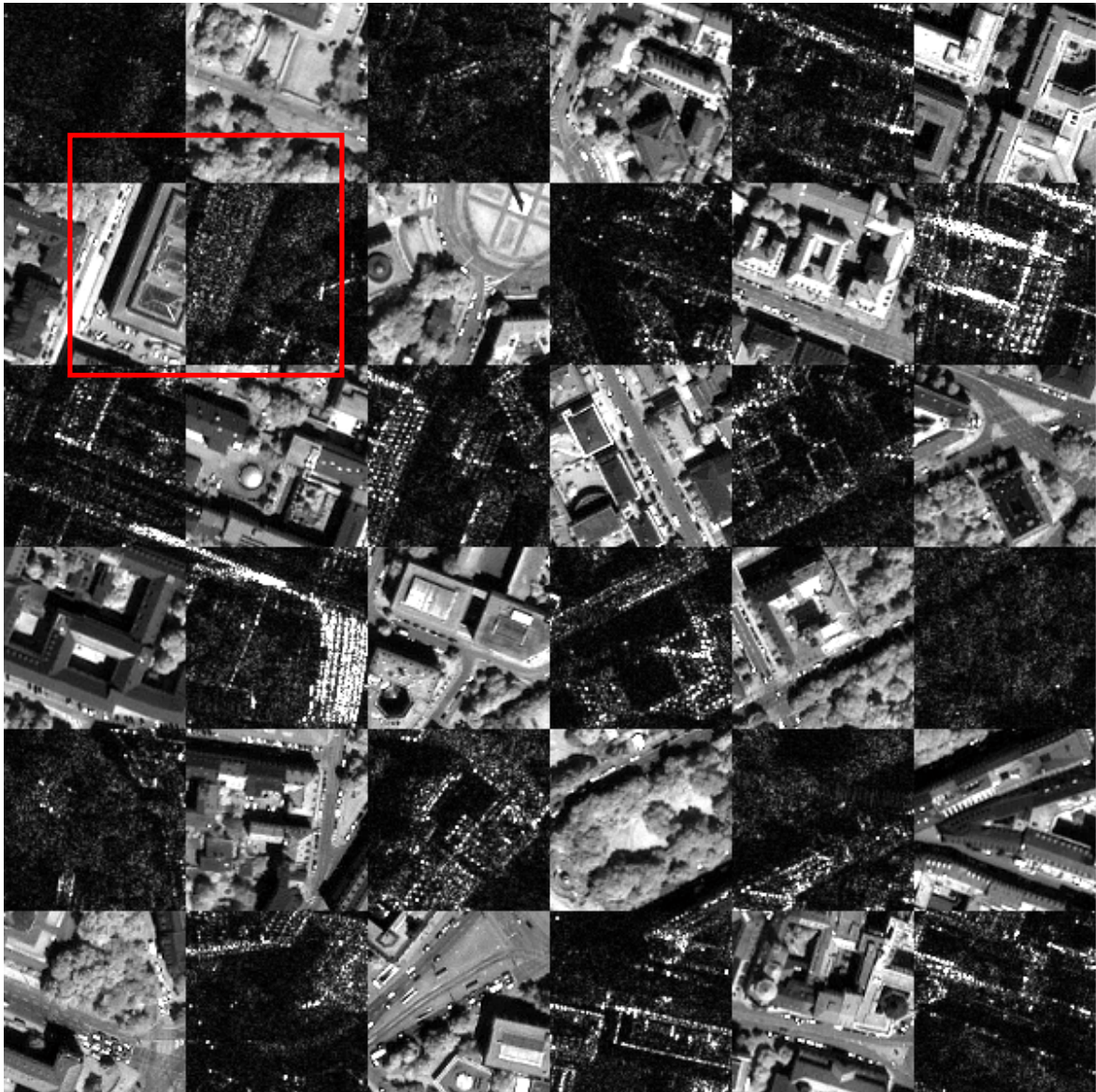
Figure 5.31: Check squared TerraSAR-X and IKONOS image orthorectified through improved sensor orientation. As in Figure 5.30 we observe good registration of “on ground” features but the highlighted flat roof building shows a misalignment. Image area is of size 600x600 pixels and is displayed without any zoom.
