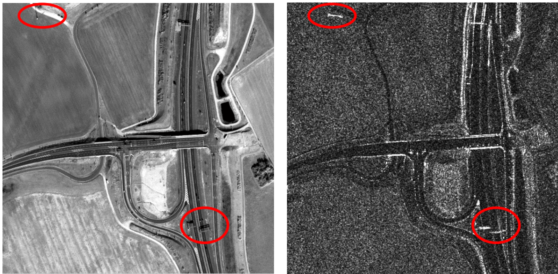
Figure 4.2: IKONOS-2 (left) and TerraSAR-X (right) imagery. Some of the objects producing incompatible response to the two sensors and should not be participating in any registration process are highlighted.
