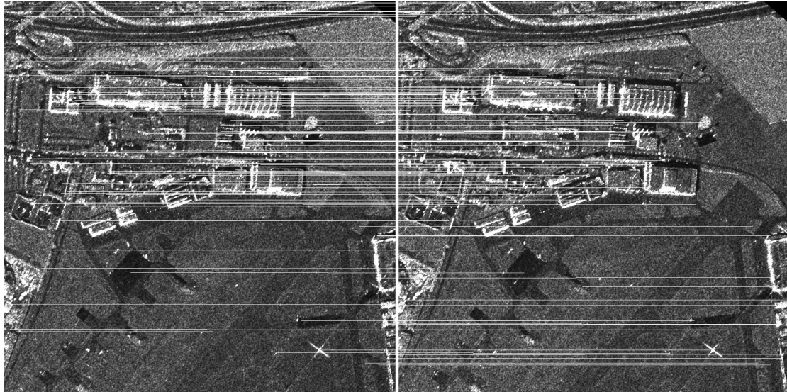
Figure 6.8: Matches found in dataset-1 after filtering them iteratively (SIFT-OCT scheme). The reference image is shown on the left, the input image on the right.
