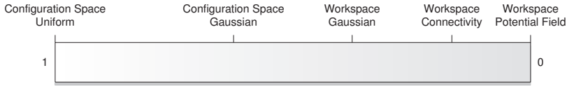
Fig. 3.12 Influence of the \sigma value in the Exploring/Exploiting Tree planner. Pure exploitation in the form of potential fields and uniform exploration in configuration space are the two extreme conditions the algorithm can achieve with a smooth transition in-between
