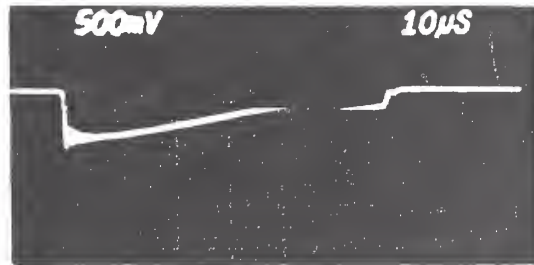
(g) voltage at box with VSP @ 25 ft. (7.5m)
