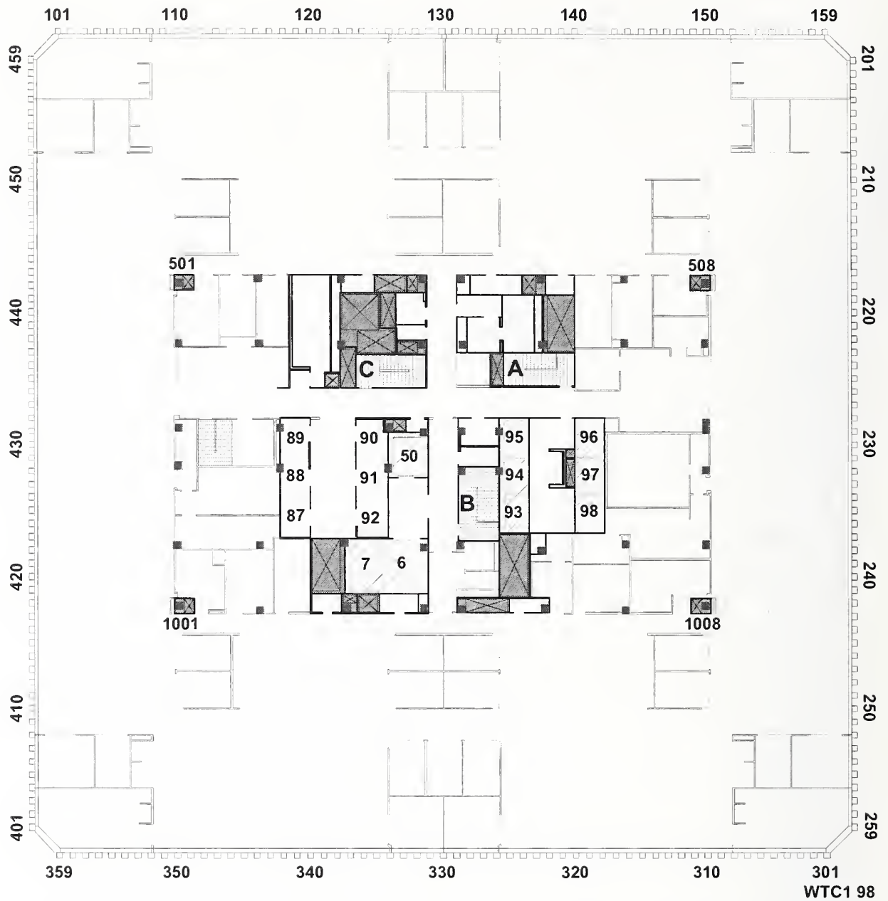
Figure B-7. This drawing shows the floor plan layout for the 98th floor of WTC 1.
