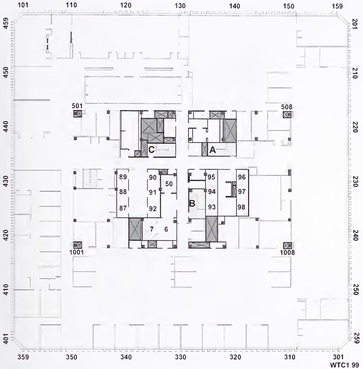
Figure B-8. This drawing shows the floor plan layout for the 99th floor of WTC 1.
