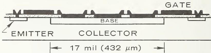
Figure 2. Cross-sectional view of the base-collector diode used for the junction C-V measurements of dopant density.
