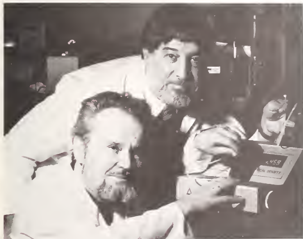
William L. McLaughlin (top) and Branislav Radak with the optical waveguide dosimeter.
