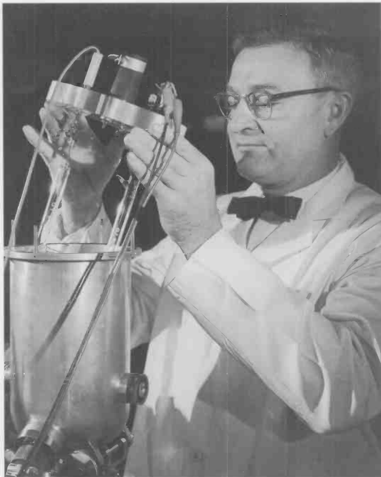
Karl F. Nefflen of the Engineering Metrology Section assembled a krypton-86 lamp. The lamp was maintained at the triple point temperature of nitrogen, 63 K, to improve the reproducibility of the standard wavelength.
