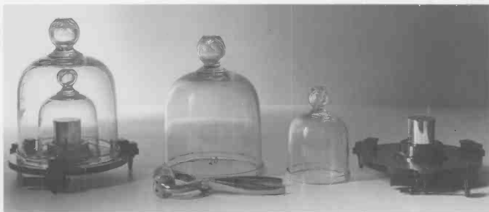
The platinum-iridium cylinder (right) is the primary standard kilogram for all metric measurements of mass in this country. Known as Kilogram No. 20, it is a copy of the international prototype kilogram, which is preserved at the International Bureau of Weights and Measures (BIPM) at Sèvres, France. Kilogram No. 4 (left, under double bell jar), a duplicate of No. 20, is used as a secondary standard.
