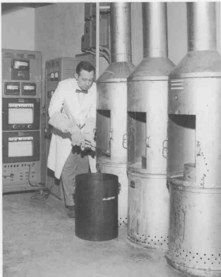
Melvin R. Meyerson of the NBS Metallurgy Division removed type 52100 tool-steel gage blocks from a chloride bath where they were immersed at 1550 °F for 15 min.
