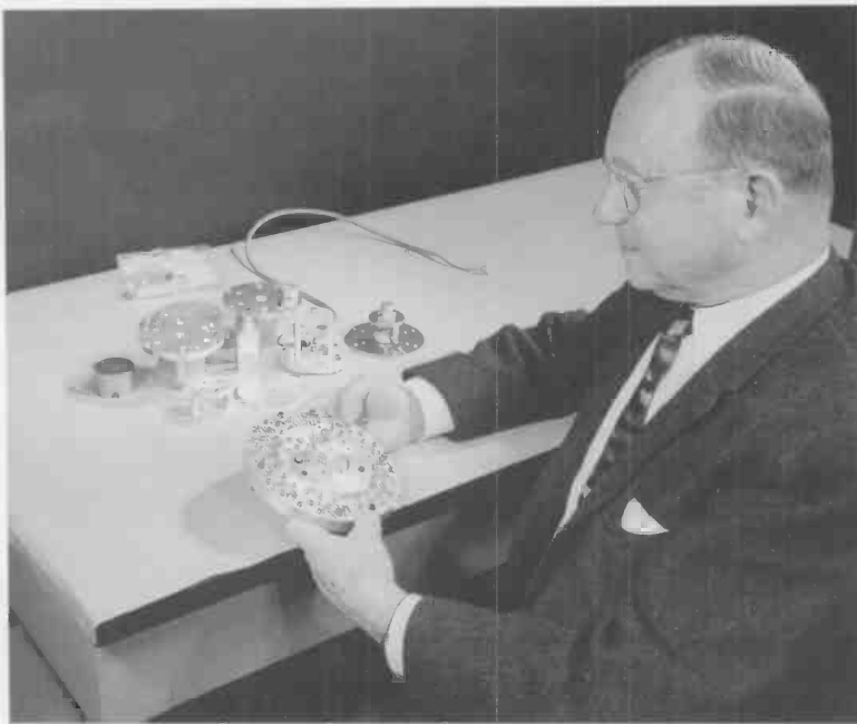
Myron C. Selby held the bolometric voltage and current (Bolovac) standard which he invented in 1967 to provide known voltages and currents at high and microwave frequencies to 20 000 MHz.
