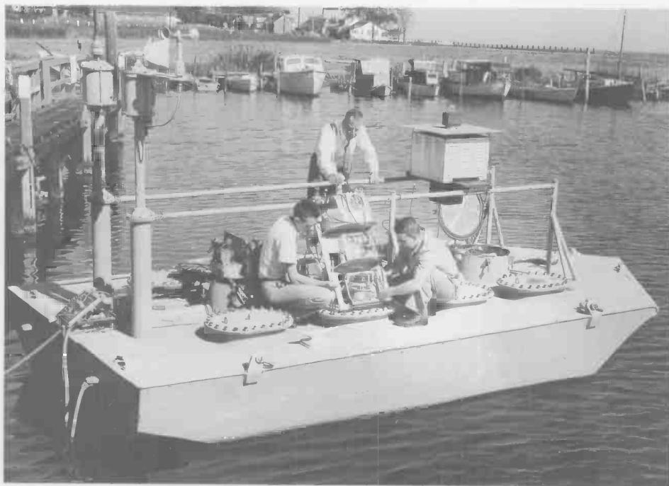
This ocean-based weather station developed by NBS automatically reported local weather data by radio. It could be anchored in a remote location and left unattended for as long as six months.
