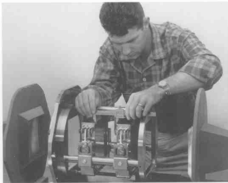
A Fabry-Perot interferometer, designed to operate at 3 mm to 4 mm, was used as the cavity resonator for a hydrogen cyanide gaseous maser. G. L. Strine was photographed in 1961 adjusting the parallelism of the perforated reflectors.
