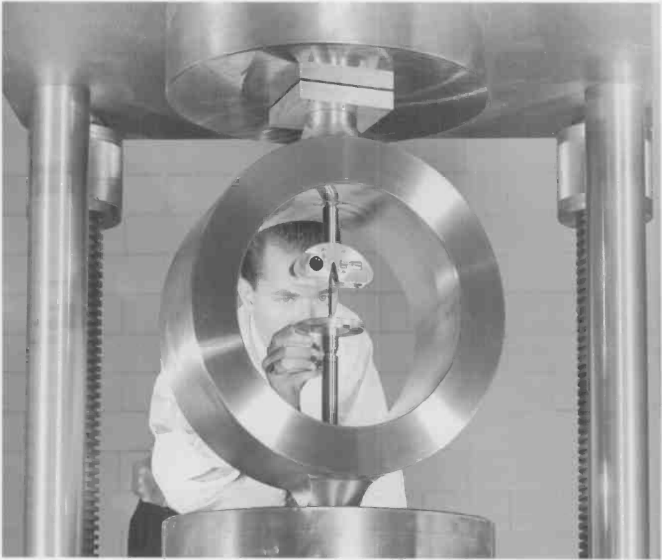
Arnold J. Mallinger calibrated a million-lb capacity proving ring in the 1-million-lbf capacity deadweight machine.
