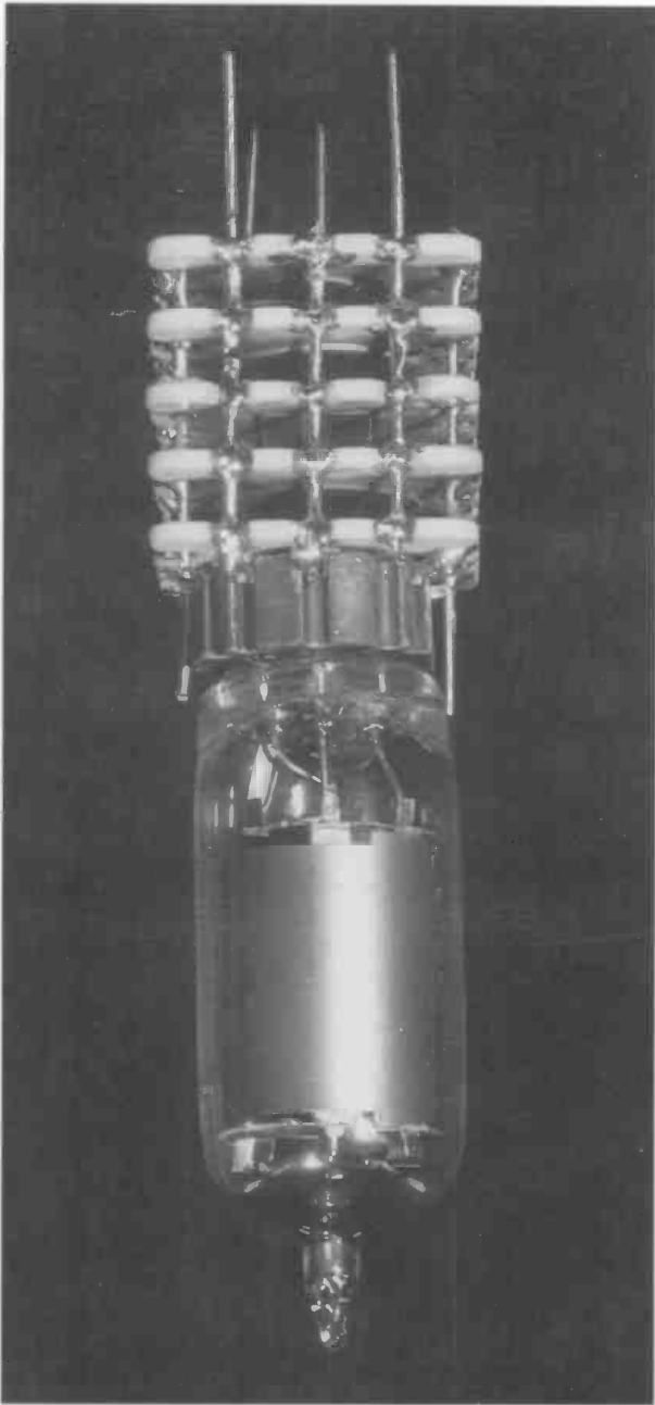
The Project Tinkertoy module. Each module was composed of four to six wafers bearing printed conducting circuits, tape resistors, capacitors, tube sockets, and other miniaturized electronic component parts.
