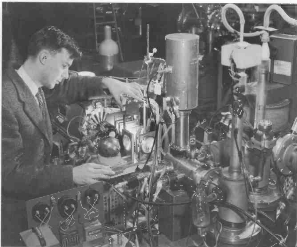
Lewis M. Branscomb inserted a filter into the optical system of the apparatus developed at NBS for studying the photodetachment of electrons from negative atomic and molecular ions (1961). The studies had direct bearing on ionospheric theory and research and on the study of plasmas.
