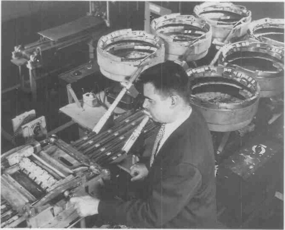
Robert L. Henry, Project Tinkertoy leader, adjusted a stencil screen mounting on the MPE wafer pattern printer.
