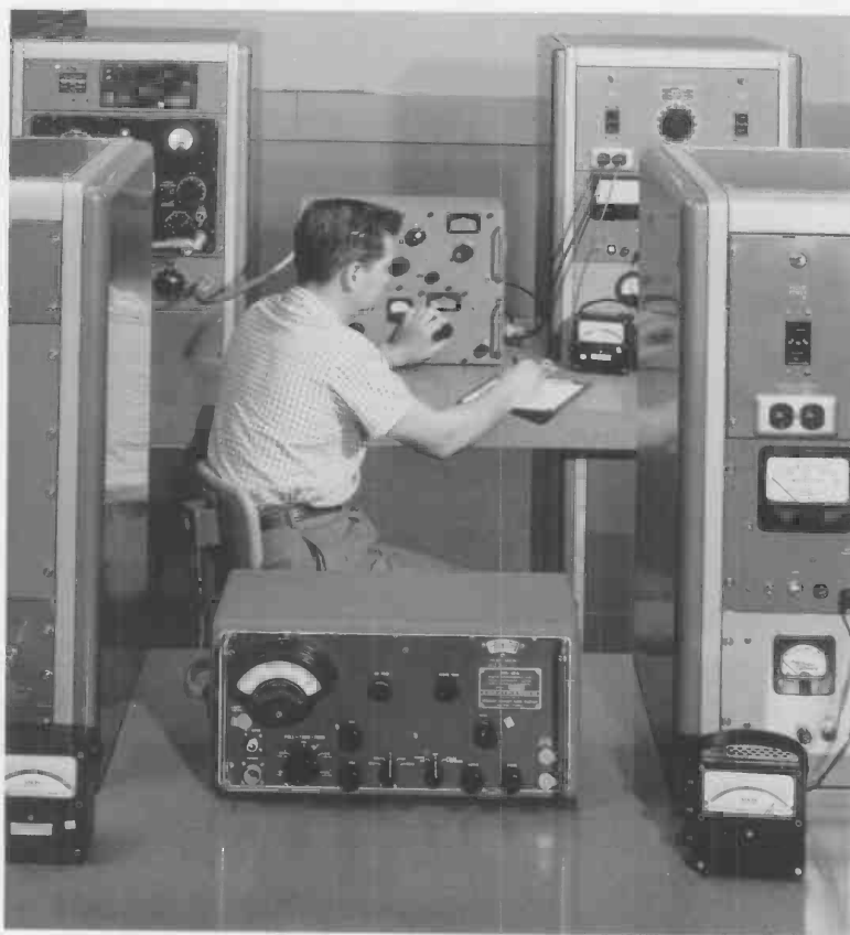
A Bureau scientist makes attenuator and linearity calibrations on a high-frequency field-strength meter.
