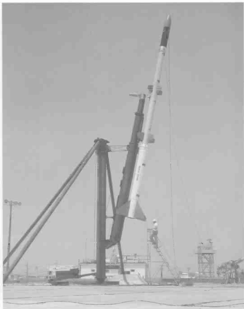
Four-stage Javelin rockets were used to carry instrumentation above the ionosphere in suborbital tests of topside-sounding satellite payloads.
