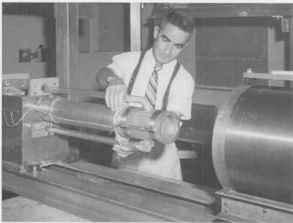
Raymond L. Driscoll with the apparatus he and Peter L. Bender used to redetermine the gyromagnetic ratio of the proton in 1958. The solenoid (center) whose magnetic field could be precisely calculated from its known dimensions, caused the protons in a water sample to precess with an accurately measurable frequency. The proton gyromagnetic ratio was then calculated from the precession frequency and the precisely known field strength. The large coils which surrounded the apparatus counterbalanced the earth's magnetic field.
