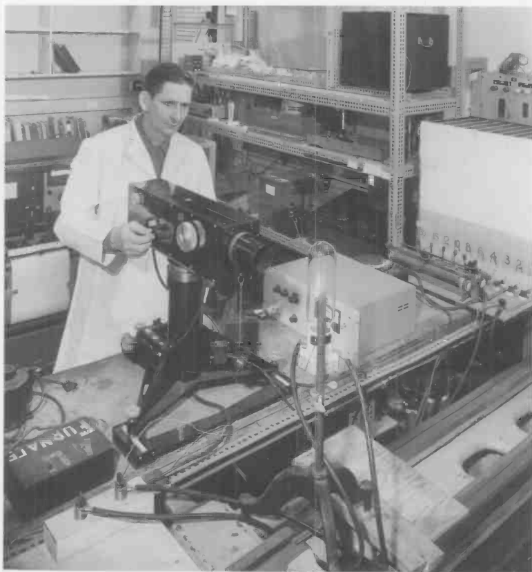
Richard Lee of the Heat Division calibrated a photoelectric pyrometer using a tungsten filament strip lamp. The tool, designed to measure the temperature of a jet engine, replaced the less accurate optical pyrometer.
