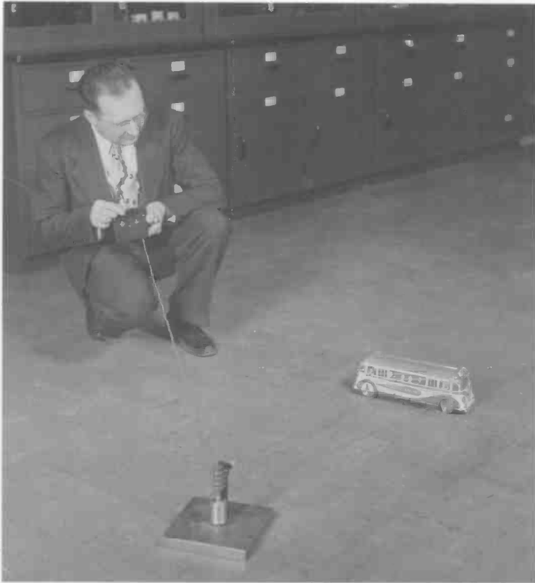
This model auto bus, equipped with a magnetic fluid clutch and a magnetic fluid brake, was constructed at NBS to demonstrate the potential application of the magnetic fluid principle to automobile clutches. Jacob Rabinow, inventor of the clutch, operated the model.
