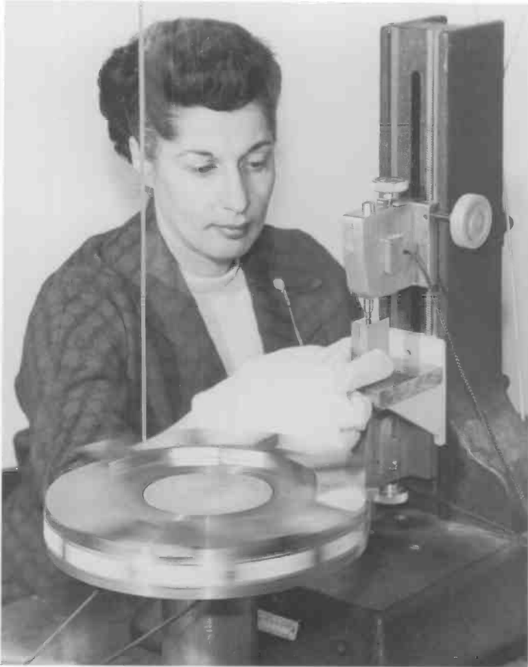
Grace Chaconas of the NBS Optics and Metrology Division positioned a pair of gage blocks in a mechanical comparator. Such comparisons, carried out in accordance with a specially designed statistical procedure, provided data on the stability of gage blocks being developed by the Bureau.
