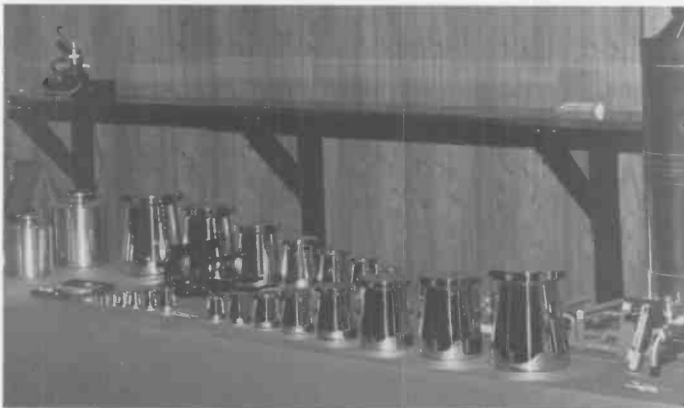
A portion of the 67 mass standards (metric and avoirdupois) presented to the State of Maryland are shown here.
