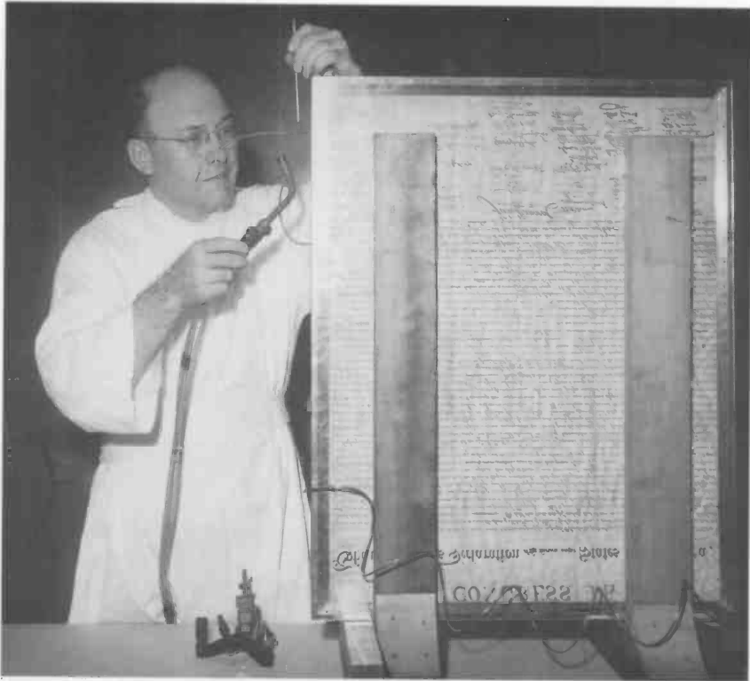
Copper tubing which led from a pure helium source was connected to the inlet tube of the test enclosure containing the Declaration of Independence in order to flush all air from the assembly. E. Carroll Creitz sealed the joint on the enclosure after the air had been completely removed.
