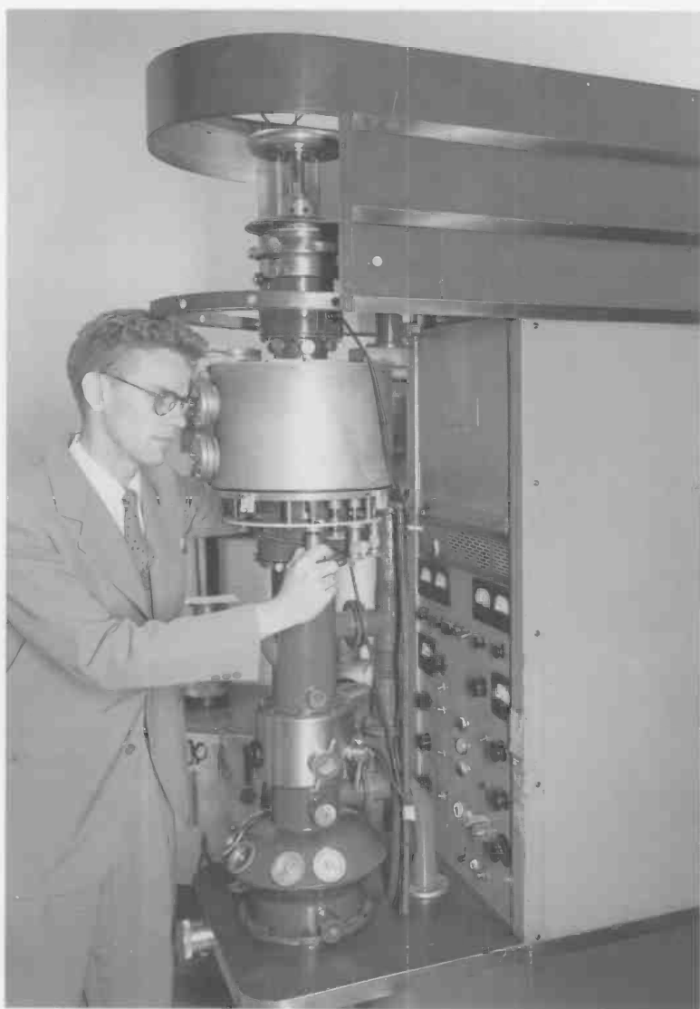
John Simpson adjusted an electron-beam interferometer, a device that utilized electron beams to produce interference fringes in much the same way that conventional optical interferometers used light beams. The instrument employed diffraction from an extremely thin crystal as a means for splitting and recombining an electron beam. Three crystals were mounted in a vacuum chamber (center) placed between the illuminating and viewing systems of a conventional electron microscope. Each of the crystal mounts could be rotated around the optical axis. The mount of the first crystal could also be translated along the optical axis. The controls for these motions were brought out at the bottom of the evacuated chamber.
