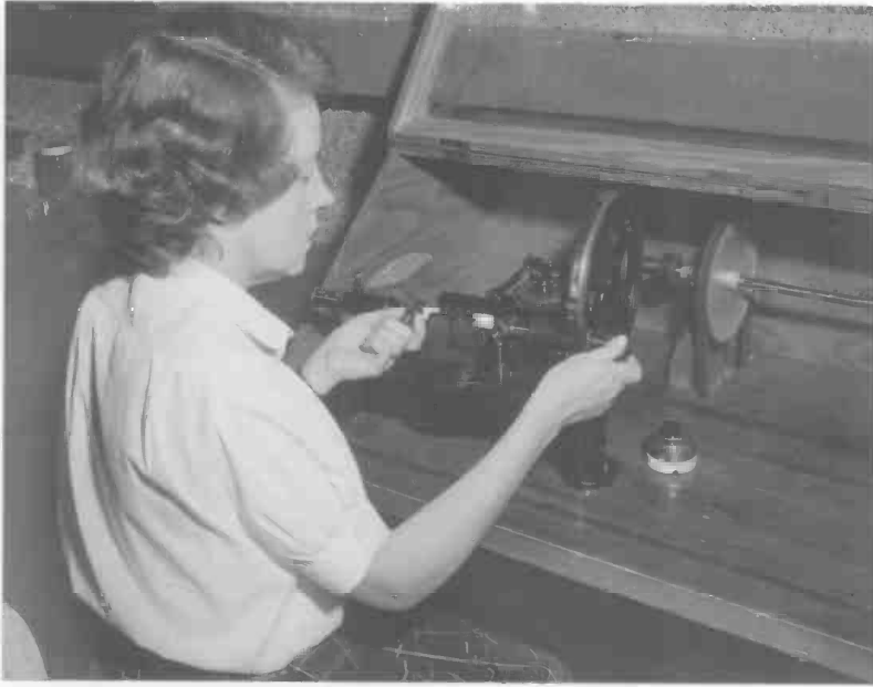
Thelma Worksman measured the folding endurance of a paper specimen. The specimen was alternately folded, under 1 kilogram tension, in opposite directions until failure occurred. The number of folds until failure was indicated on the small horizontal wheel behind and right of the specimen. Statistical analysis of the Bureau's data on folding endurance showed a fair correlation between natural and accelerated aging.
