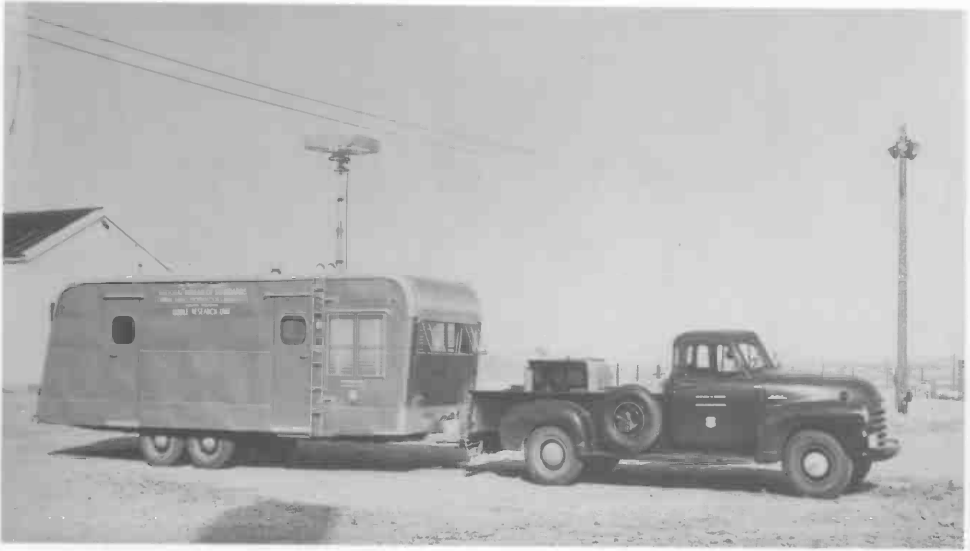
Mobile research unit used by NBS to measure the field strength of radio signals. The antenna on top of the trailer could be raised to a height of 30 ft by remote control while the unit was in motion.
