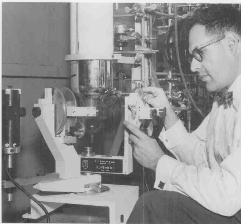
Jerome Kruger, metallurgist on the Bureau staff, demonstrated an ellipsometer to study corrosion reactions on the surfaces of metal single crystals. The instrument was on display during a two-day symposium on ellipsometry held at the Bureau in September 1963.
