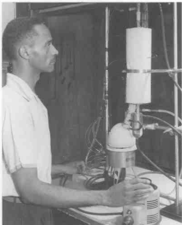
This high-temperature drop calorimeter was used in studies of the excess entropy of glass by Cornelius Pearson as he measured the vapor pressure of arsenic oxide in the crystalline and vitreous states to determine entropy of vaporization.
