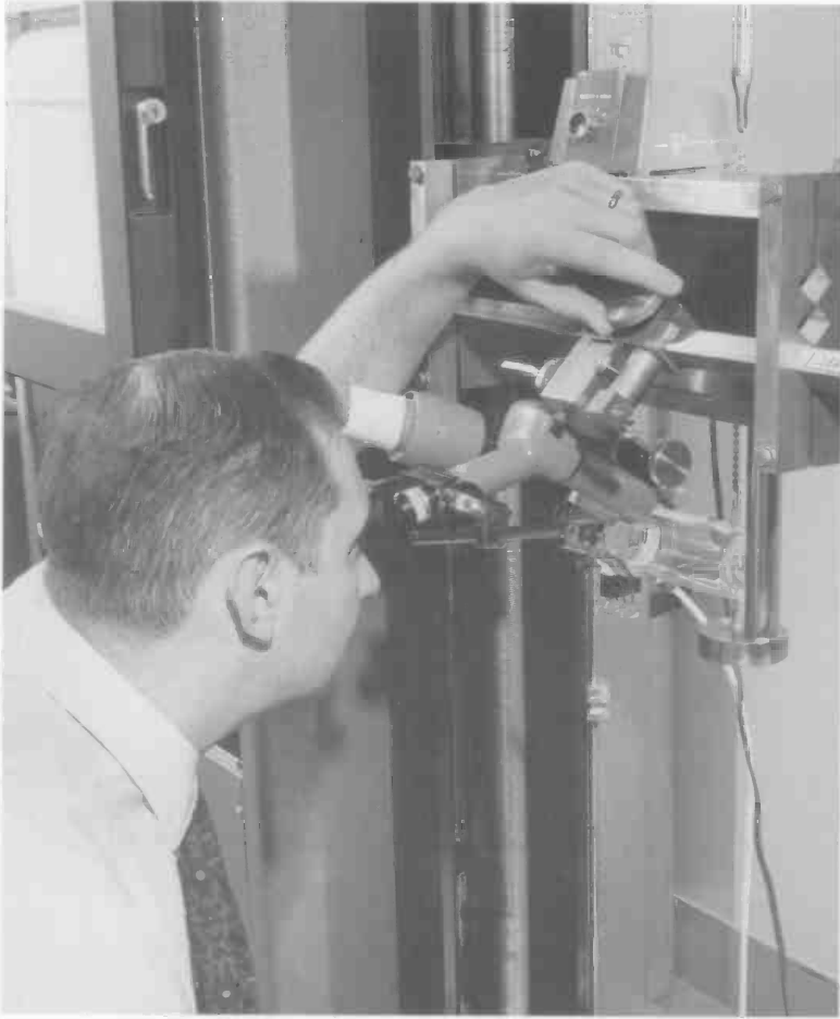
Sheldon M. Wiederhorn observed the motion of a crack in a soda-lime glass with the aid of a traveling microscope. The specimen, a microscope slide, could be seen within the environmental chamber with two hooks attached to one end. The hooks, in turn, were attached to the jig of a testing machine that applied a stress to the sample. At the same time, a continuous stream of the desired atmosphere entered the test chamber by way of the white tubing in the background.
